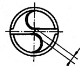
Chisel edge length 10% of the drill bit - Ø
