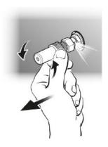
Fig. 9: Safety valve with ring nut
