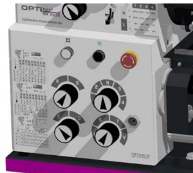
Img.4-2: Selector switch infeed
