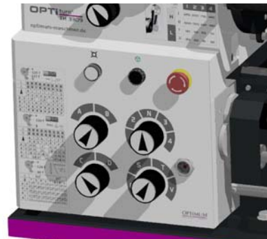
Img.4-3: Selector switch infeed
