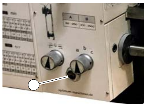
Feed gear inspection glass
