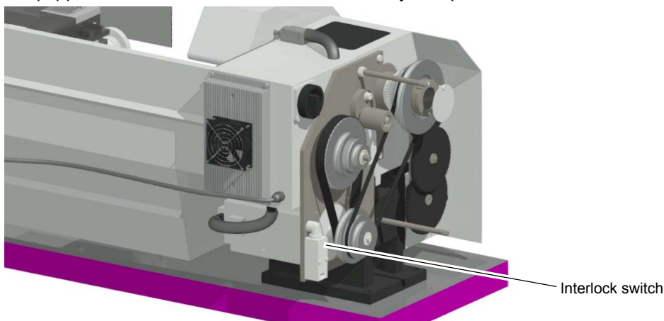
Img. 1-2: Protective cover of the headstock
