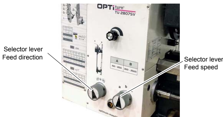
Img.4-6: Changing the feed rate
