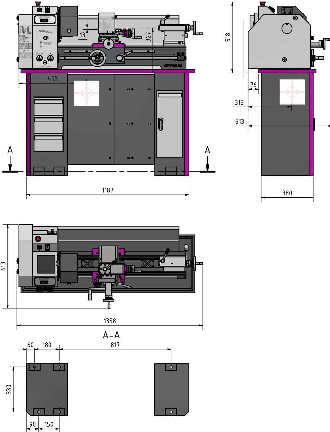
Img.3-1: Floor fixing
