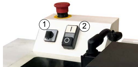
Rotation direction switch (1) On / Off switch (2)
