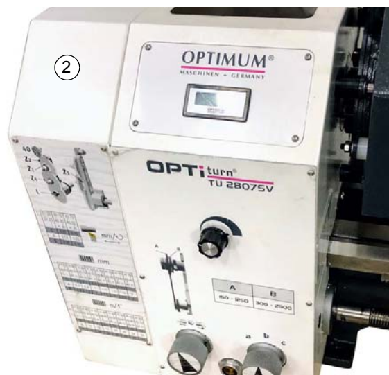
Img.4-2: Protective cover of the headstock
