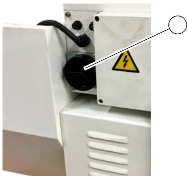
lockable main switch
